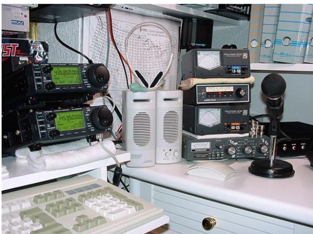
Photo n°3: A couple of IC-706MKIIG transceivers, one for UHF and the other for VHF, both of them computer controlled by of the CAT port and the software, working the satellite.
